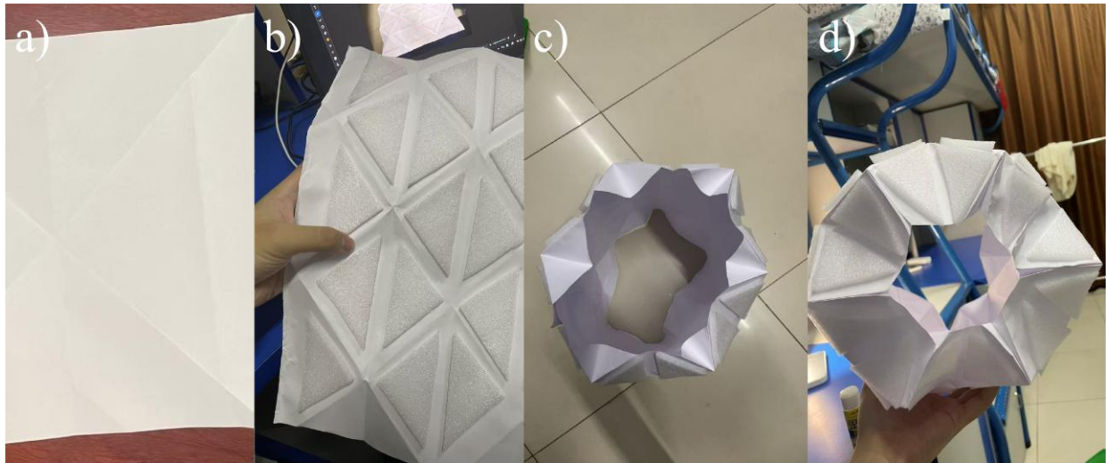
Figure 4. Fabrication Process of the Paper-based Wrapping Structure Based on the Origami Principle: a) Creating creases on the paper b) Cutting and bonding of foam units c) Crease pre-treatment and three-dimensional structure formation d) Squeezing and final formation of the wrapping structure.
