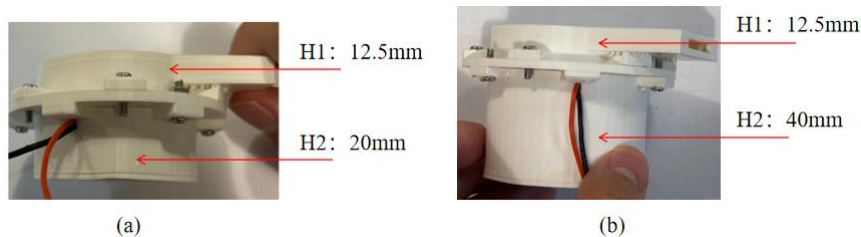
Figure 10. Different back cavity SPK modules: (a) type 1-2; and (b) type 2-2
