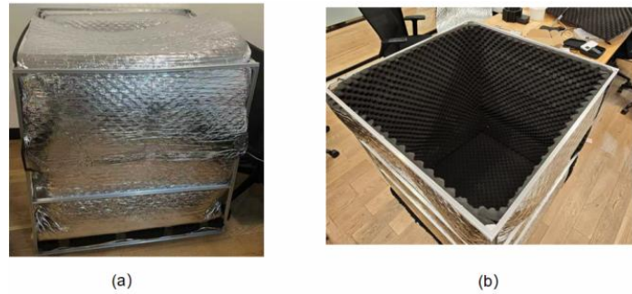
Figure 3. Square anechoic chamber: (a) outer structure; and (b) inner structure.
