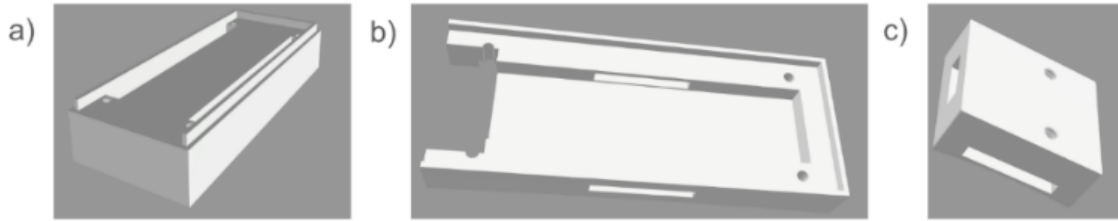
Figure 8. The 3D printing model of the holder and caps for the vibration motors and esp32 board.
